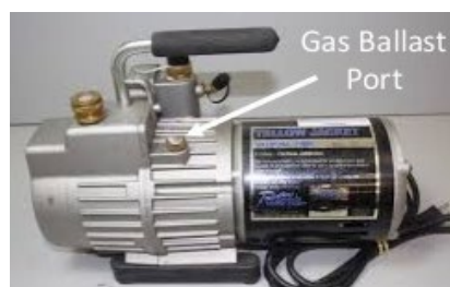
Figure 8.23. Yellow Jacket pump showing location of gas ballast port.
