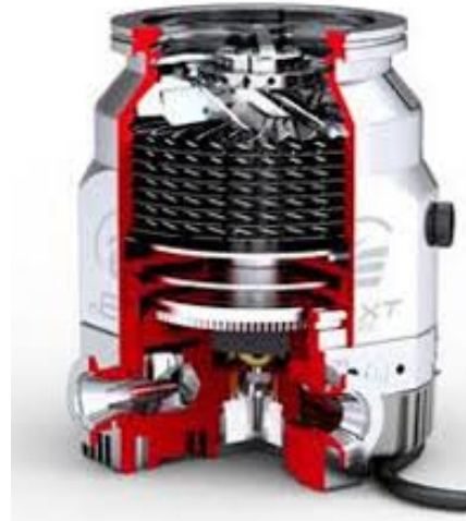
Figure 8.17. Cut away showing both turbomolecular and drag stages within a turbodrag vacuum pump.
