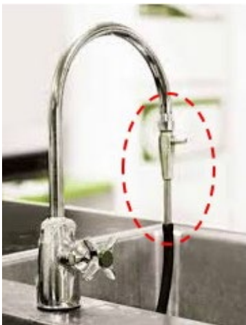
Figure 8.7. Water-driven aspirator vacuum pump - historically used in high-school chemistry classes.
