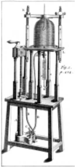
John Smeaton (1724 -1792 ) Improved air pump and “Pear” vacuum gauge 1/1000 atm 1751
