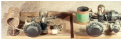
Complete amateur radio station 1-tube receiver and 1-tube transmitter 1929
