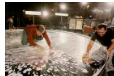
200-inch Mt. Palomar telescope mirror coated by aluminum evaporation from 350 tungsten filaments (mirror cleaning c. 1997) John D. Strong 1947
