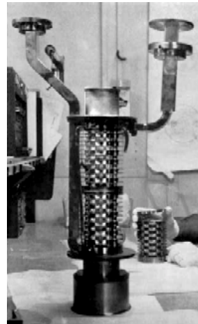
Varian VA-126 High-power traveling wave tube 1962
