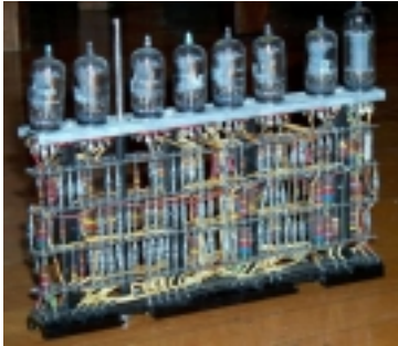
IBM 709 computer Last major vacuum tube computer Magnetic core memory 1958
