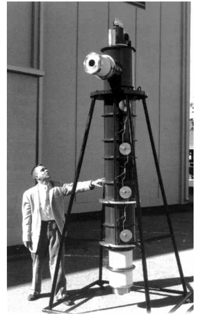
Varian Klystron (VA-842) Liquid-cooled, multicavity radar transmitting tube - the largest documented production klystron 1959
