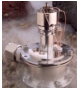
The world's smallest high- performance quadrupole mass spectrometer (16-rods) installed in the International Space Station 2001
