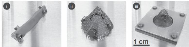
**Fig. 2. Examples of cage styles used for etching are (l-r) triangular with fine mesh; wrapped with course mesh; molded with medium mesh.**
