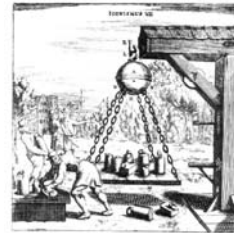
Fig. 3. Hermann Nill (from von Guericke's book of 1672). Atmospheric pressure measured copper hemispheres apart by applying weights. (Courtesy of the "Otto-von-Guericke" University, Magdeburg, Germany.)
