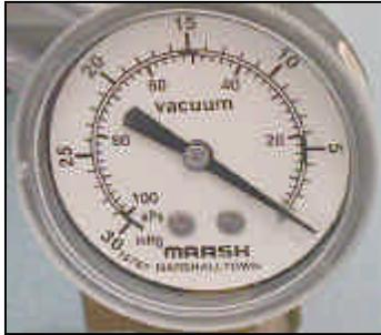
Vacuum gauge reading atmospheric pressure
