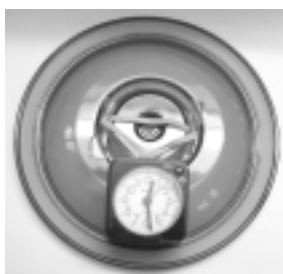
Rubber band taped to clock and inside of canister lid
