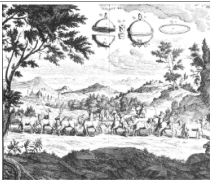
Demonstration of air pressure at Magdeburg, Germany 1657. Probably first demonstrated in 1648 by Otto von Guericke.
